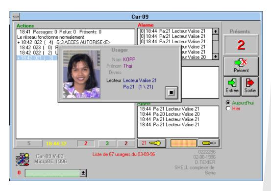
The Car-09 acquisition module memorizes with timestamp all actions carried out in the network, as well as the accesses and the input status changes.
