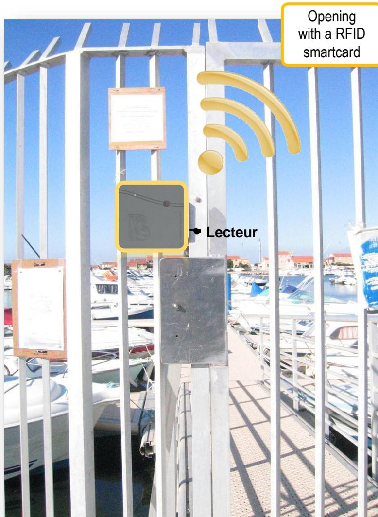
Thanks to its standalone function, a system with multiple control points can be created. The reader's intelligence and the information contained in the card is used to make decisions locally without using a cabled network.
